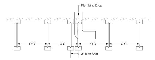
If a shift greater than 3" is needed, and additional joists are impractical, Pinkwood recommends "heading out" the joist and creating a double joist header as depicted in detail 1h below from Pinkwood's Install Guide. Please contact customer support with any questions or concerns.
