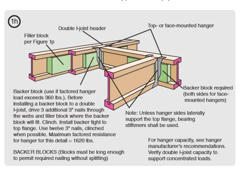
Additional analysis may be required to ensure adjacent joists can support the added loads.
