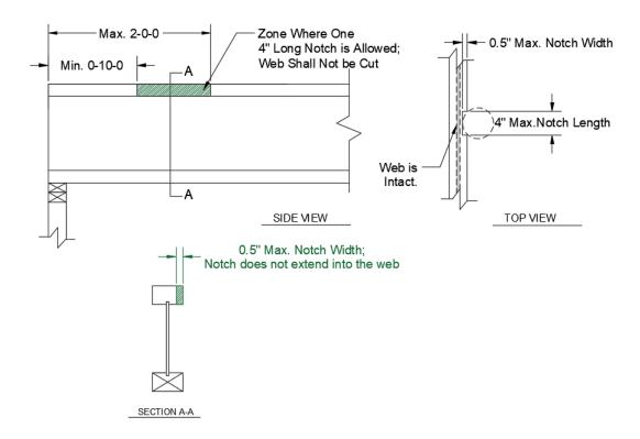
NOTE: When top flange notches are within the guidelines listed above, no repair engineering or sealed calculations are required.
