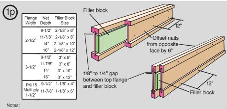
1. Support back of I-joist web during nailing to prevent damage to web/flange connection.
